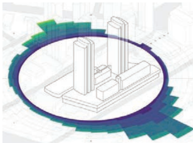
CFD Wind at 8m/s from ENE (68) Prevailing wind
