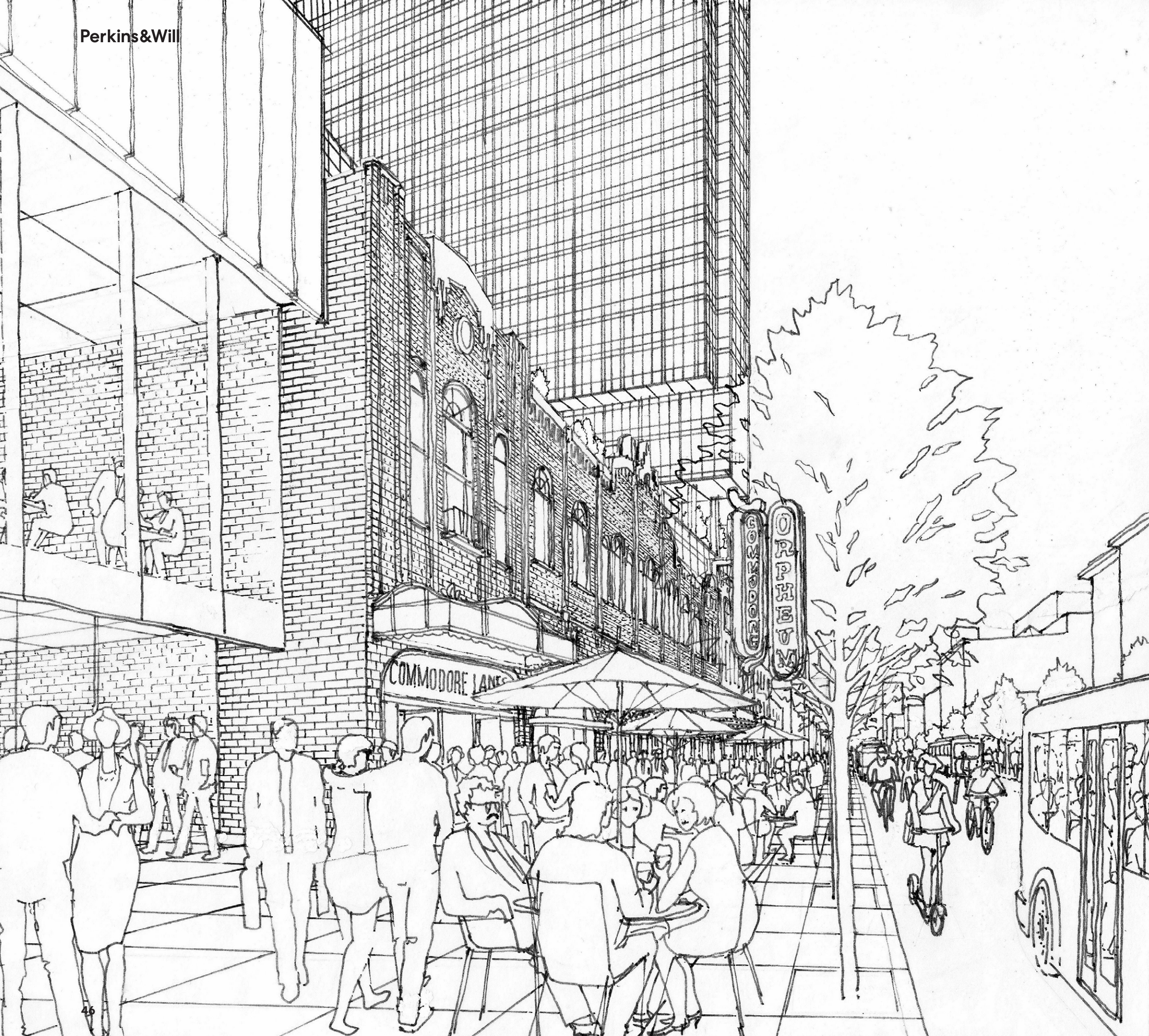
A Granville Street view showing design intent of the full preservation of the Commodore Ballroom, Lanes and Retails at ground through stepping back the new retail infill levels and announcing the prominent return of the Commodore side wall.
