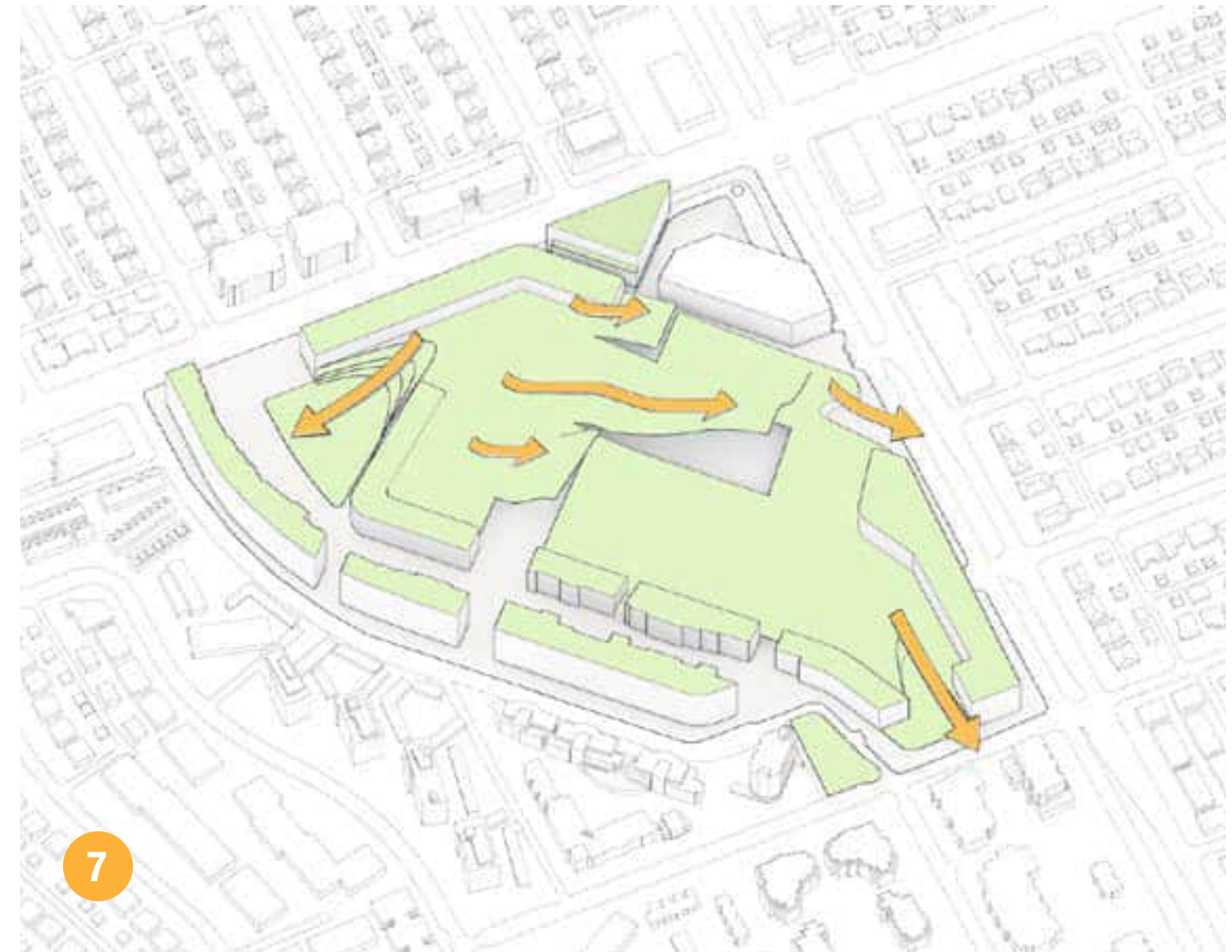
The new landscape skin is manipulated and peeled to allow light to enter the mall below and folded to transition down to grade at the edges of the site.
