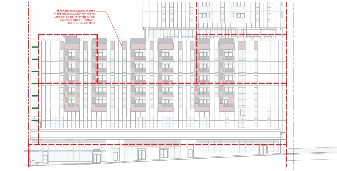
Proposed Granville Street (West) Elevation with the Rezoning Form of Development massing overlaid in Red.
