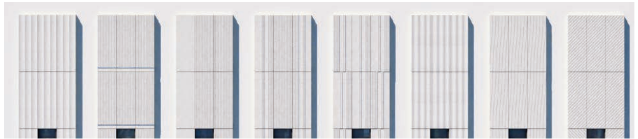
Cladding texture studies for the upper podium and tower portions of the building. Final material selection is in progress.
