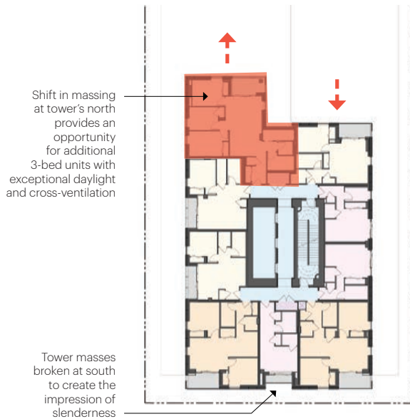
Tower floor plate shape
