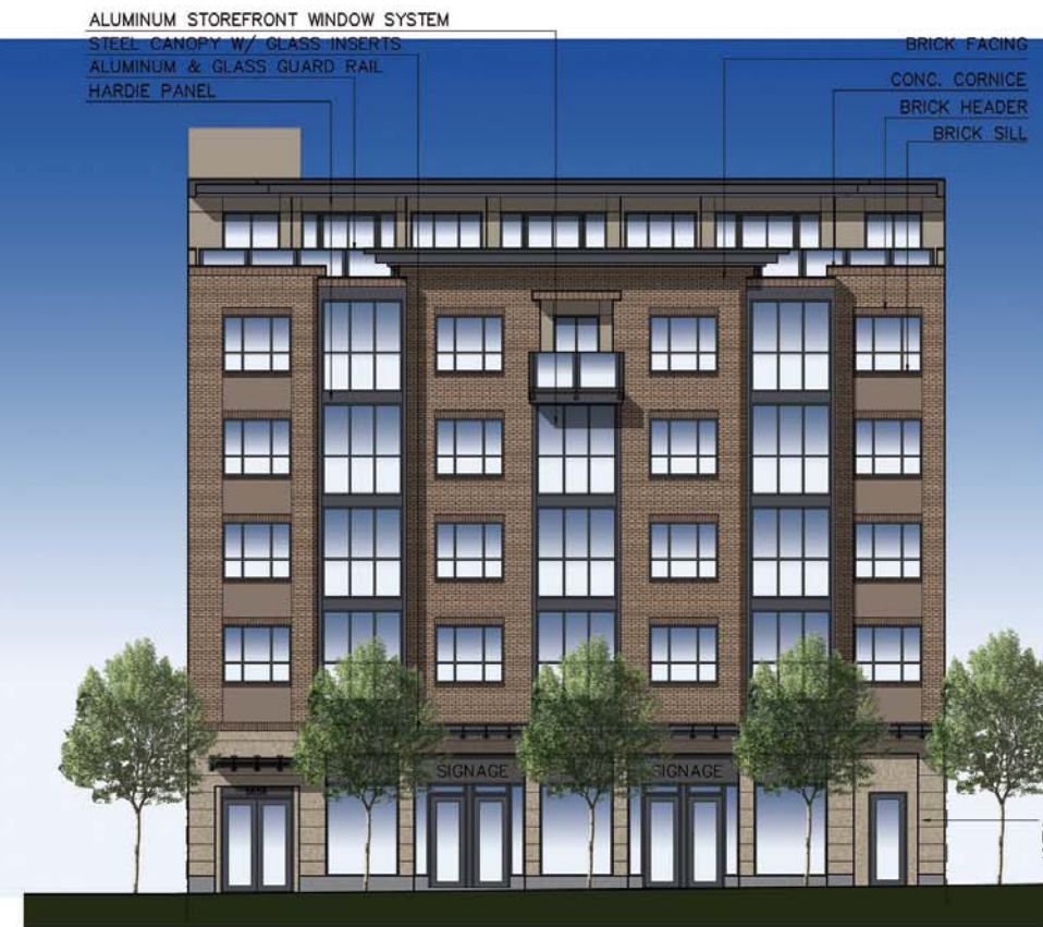
WEST ELEVATION (VICTORIA)
