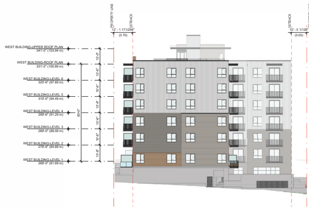
Internal Elevation - West Building
