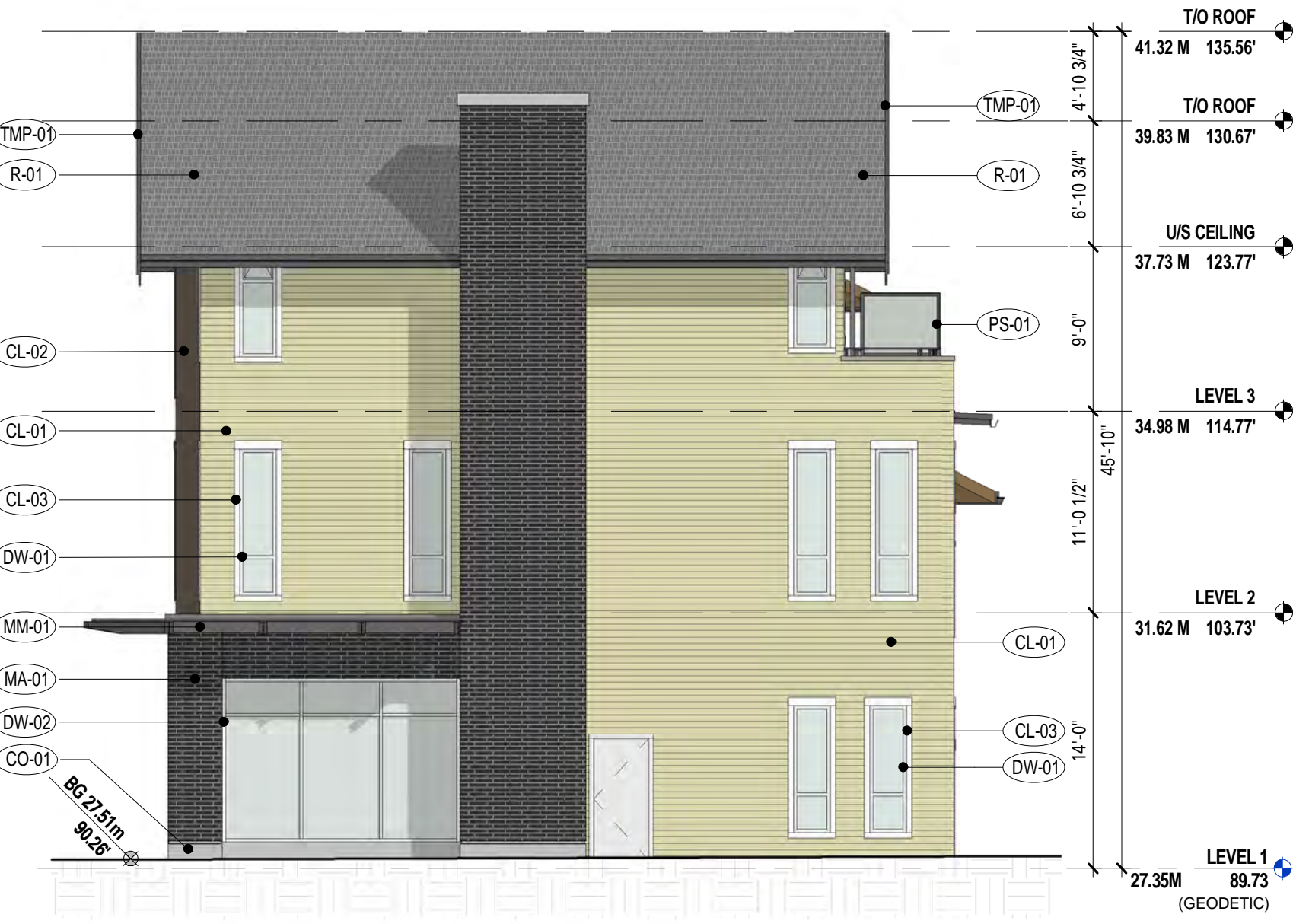
2 SOUTH ELEVATION - WEST BLDG. 1/8" = 1'-0"
