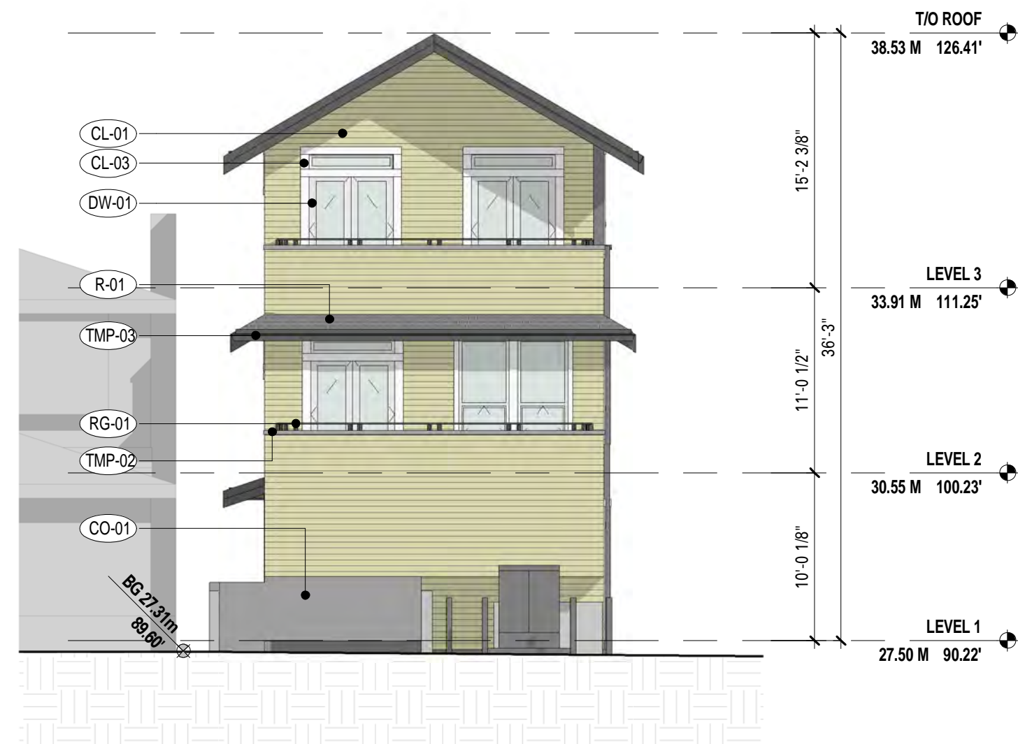
3 NORTH ELEVATION - EAST BLDG 1/8" = 1'-0"
