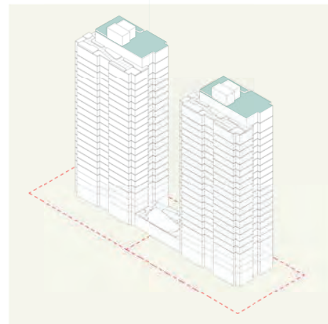
7 Extrude Elevator Room Extrude elevator rooms and provide space for mechanical equipment.
