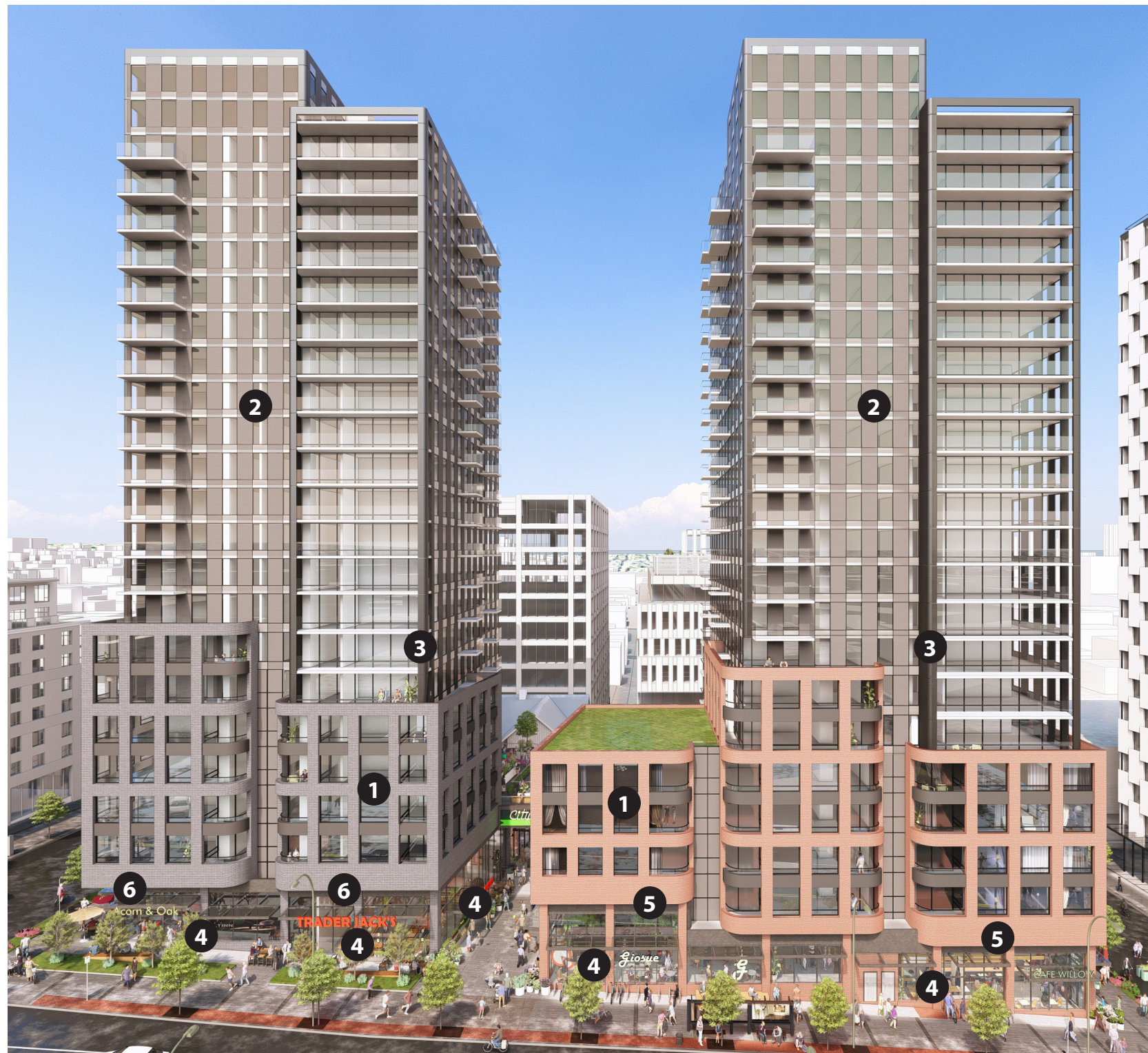
Metal Panel Window Wall System Glass: Double Glazed, Insulated
