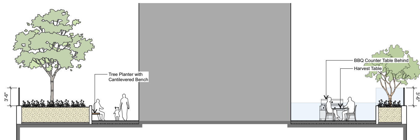
5 ROOF LEVEL TREE PLANTERS L2.01 Scale = 3/16" = 1'-0"
