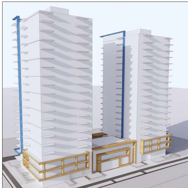
HORIZONTAL ARCHITECTURAL ELEMENTS AT PODIUM (YELLOW) AND VERTICAL FRAME ELEMENTS (BLUE) TO ACHIEVE A SCALE THAT IS RELATABLE TO STREET ORIENTED HUMAN EXPERIENCE. - NORTH
